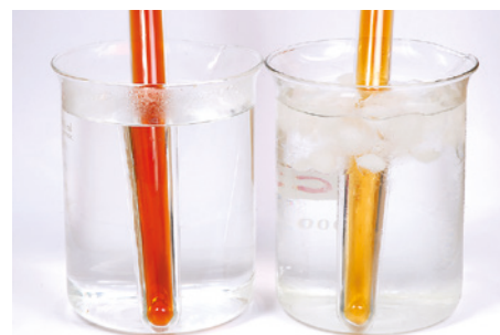
FIGURE 2.6.8 Equilibrium mixtures of \text{NO}_2 and \text{N}_2\text{O}_4 in hot water and ice. Heating the mixture favours the formation of brown \text{NO}_2 gas.
