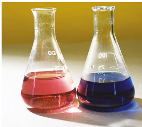
FIGURE 2.5.1 The effect of changes on the equilibrium: \text{Co}(\text{H}_2\text{O})_6^{2+}(\text{aq}) + 4\text{Cl}^-(\text{aq}) \rightleftharpoons \text{CoCl}_4^{2-}(\text{aq}) + 6\text{H}_2\text{O}(\text{l}) . The addition of excess \text{Cl}^- ions causes a net forward reaction and the solution turns blue as more \text{CoCl}_4^{2-} is formed. The addition of excess water causes a net reverse reaction and the solution returns to the original pink colour as more [\text{Co}(\text{H}_2\text{O})_6]^{2+} is formed.
