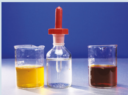
FIGURE 2.3.3 Chemicals needed to make fake blood. From left to right: a solution containing \text{Fe}^{3+} , a solution containing \text{SCN}^- , and an equilibrium mixture of \text{Fe}^{3+} , \text{SCN}^- and \text{FeSCN}^{2+} .
